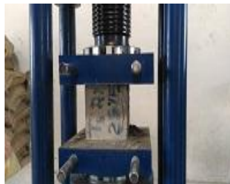
Fig 12: Testing of a Cube specimen
