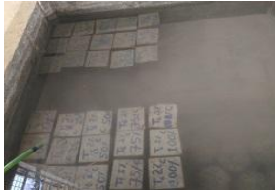
Fig 11: Curing of concrete cubes
