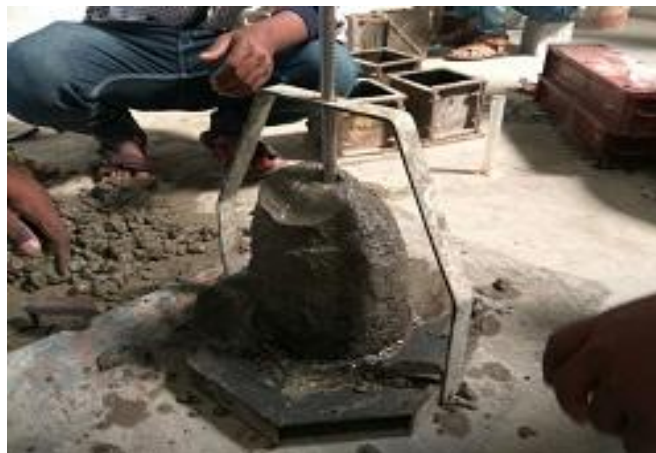
Fig 7: Slump Cone Test
