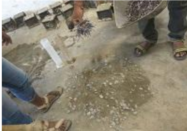
Fig 8: Addition of Steel Fibers
