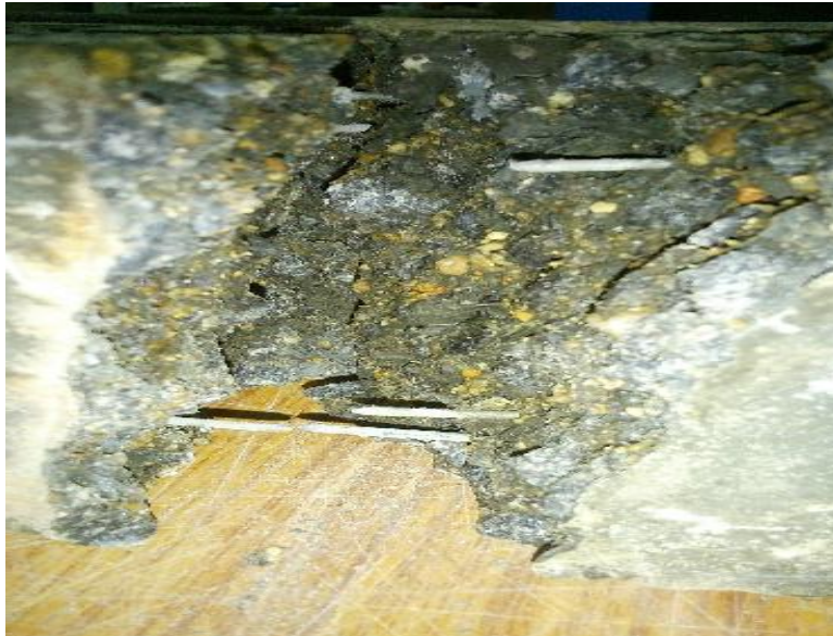
Fig5: Cup- cone failure in tendons
