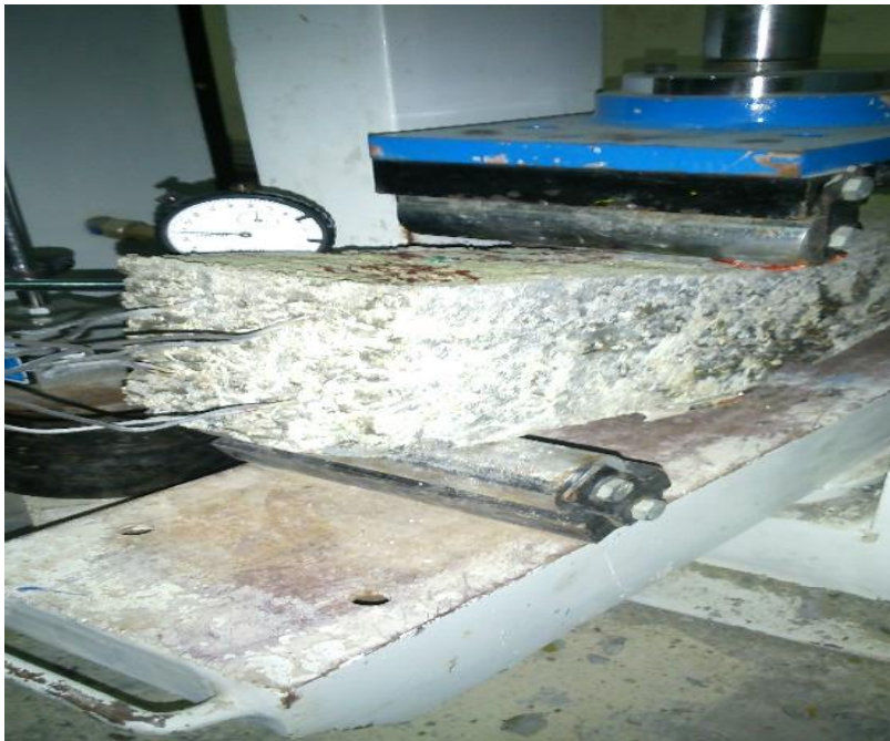
Fig4: Beam failure in flexure testing machine
