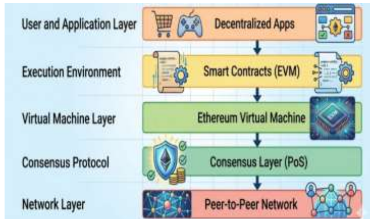
Figure 1: Ethereum Ecosystem Architecture (2D Model)
