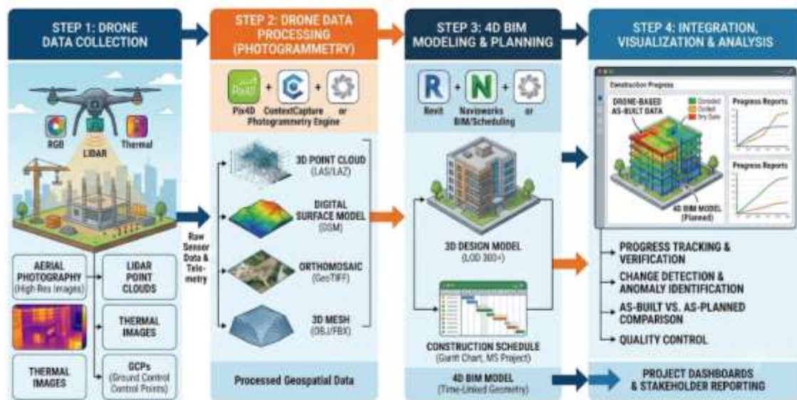
Figure 1: End-to-end technical data workflow illustrating the collection, processing, and integration of drone data with 4D BIM models
