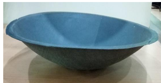
Figure 6: Cured reflector manufactured using hot air oven process
