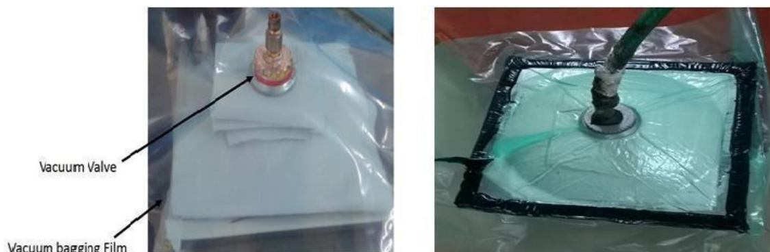
Figure 3: Vacuum bagging and air suction process
