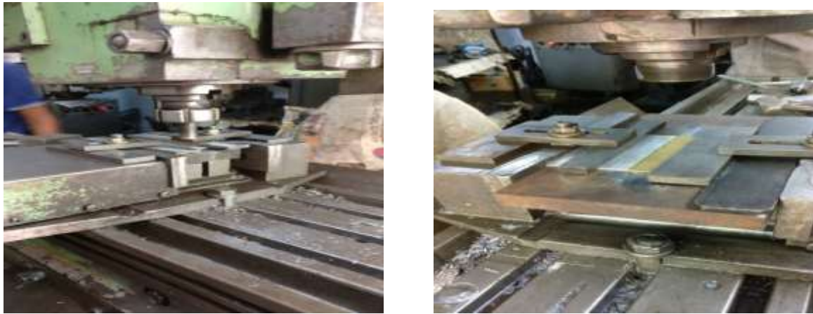
Fig 6: Experimental Setup in a Conventional Milling machine
