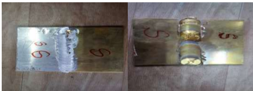
Fig7: Final Welding by using Square tool
