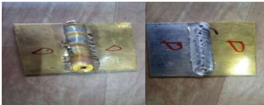
Fig8: Final Welding by using Diamond tool
