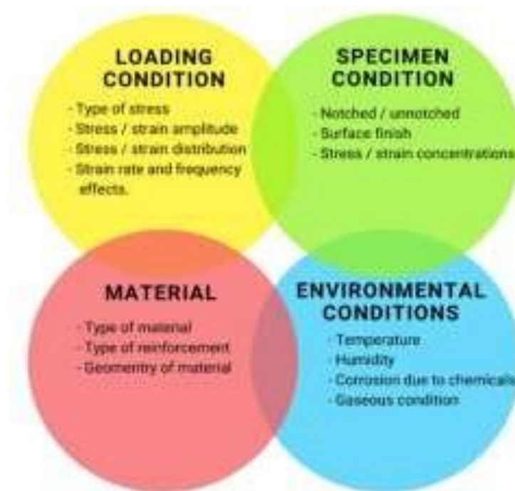
Fig.5:-Factors which effect the fatigue life of polymeric materials.
