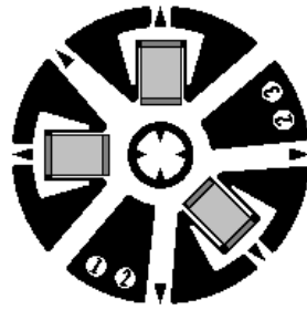
Fig:2 Strain Gage Arrangement for Measuring Residual Stress
