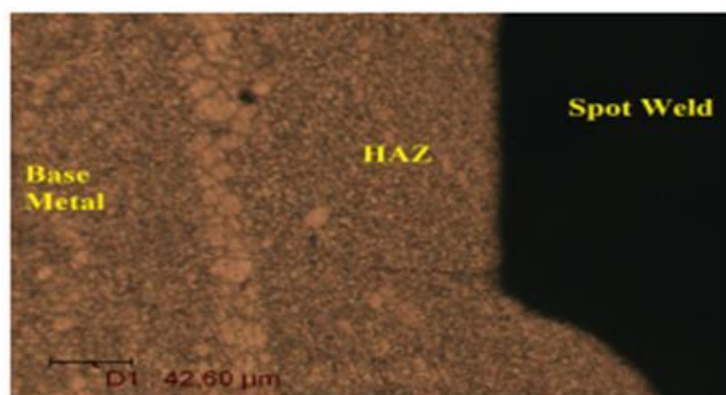
Figure 4 Microstructure of different zone in resistance spot welding
