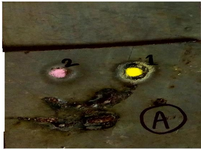
Figure 5 Failure modes in tensile test of AISI 304 resistance spot weld
