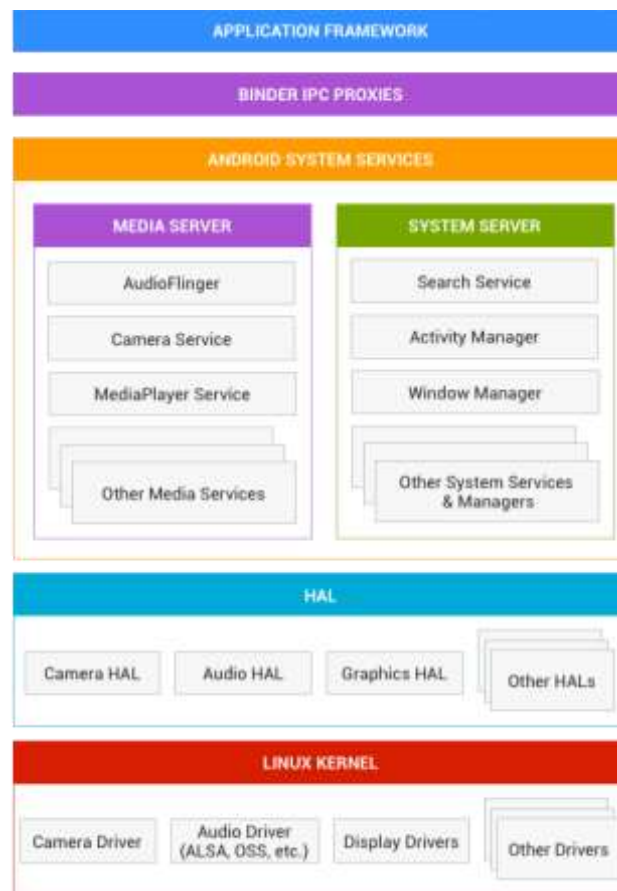
Figure 1: Android System Architecture
