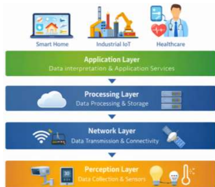
Figure 1: IoT Architecture Layers
