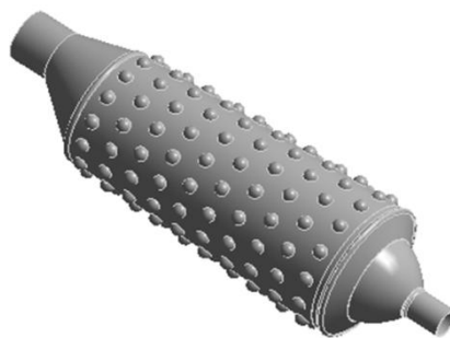
Fig. 5: Modified model having staggered dimple pattern on outer surface
