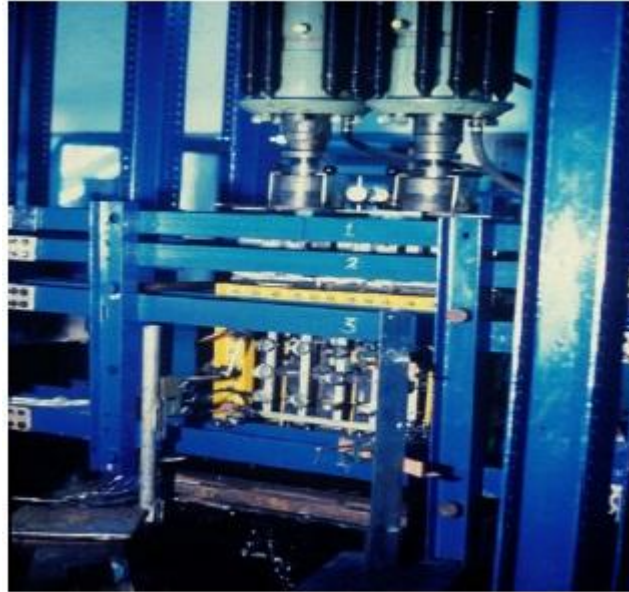
Figure 6: Stiffened Plate Model Positioned In the Ghavami's Testing Rig
