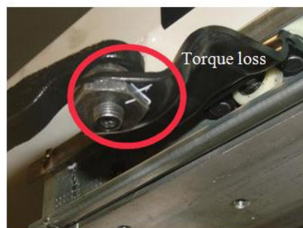
Figure: - 13 Part fails from durability test [6]
