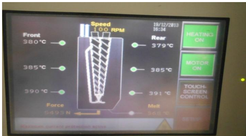
Fig. 2 Temperature profile for PEEK composites
