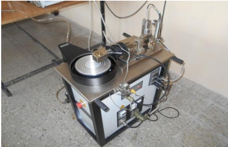
Fig. 6 Wear and friction measuring test rig TR-20
