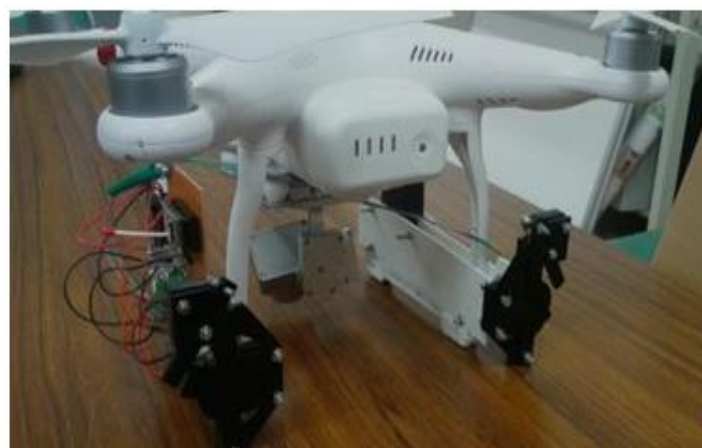
Fig.11 Gripper mounted on the ISFUAV
