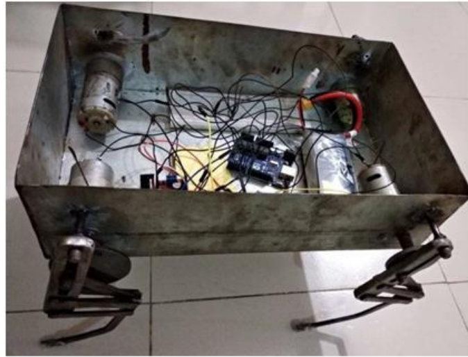
Figure 2: Four legged robot (constructed model)
