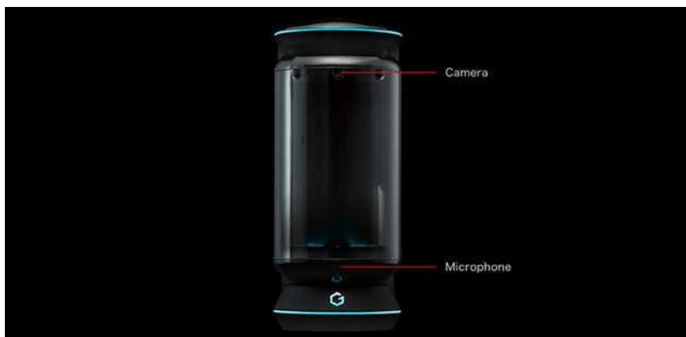
Fig.1 The virtual 3D projected home robot with camera and microphone embedded
