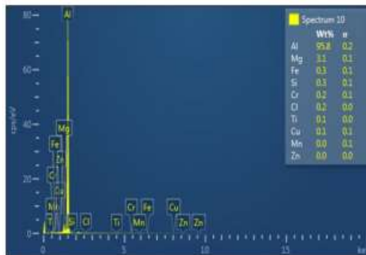
Fig.3. Chemical Composition of base materials b) AA5083
