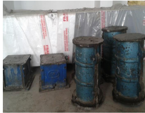
Fig 3 Casting of concrete
