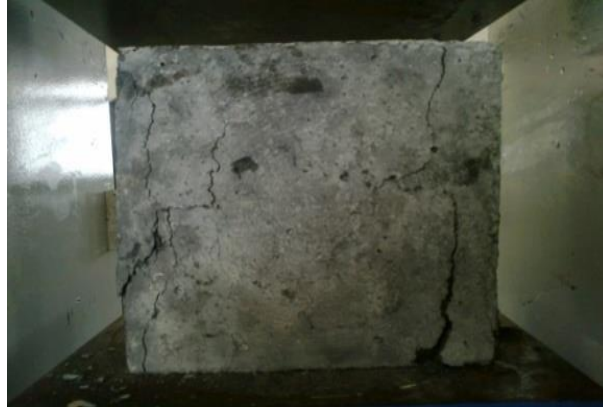
Fig 5 Testing of cube
