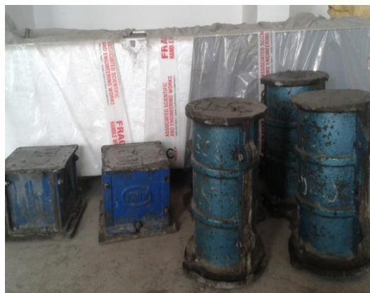
Fig 3 Casting of concrete
