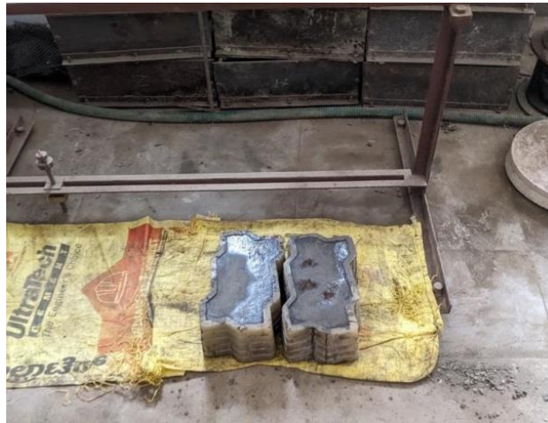
Fig 7 Geopolymer concrete in mould after 24hrs
