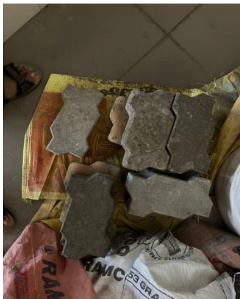
Fig 9 Curing of interlock in ambient temperature
