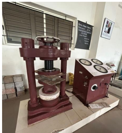
Fig 10 Compression test machine with inter lock.
