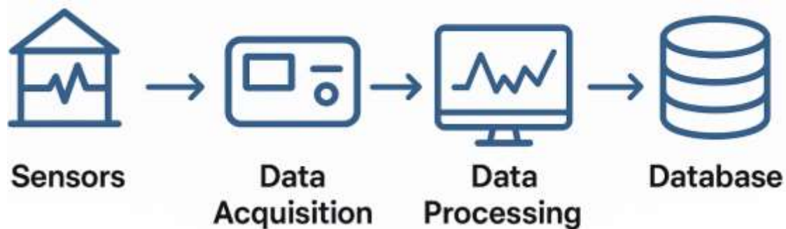
Figure 1: General Structural Health Monitoring System Architecture
