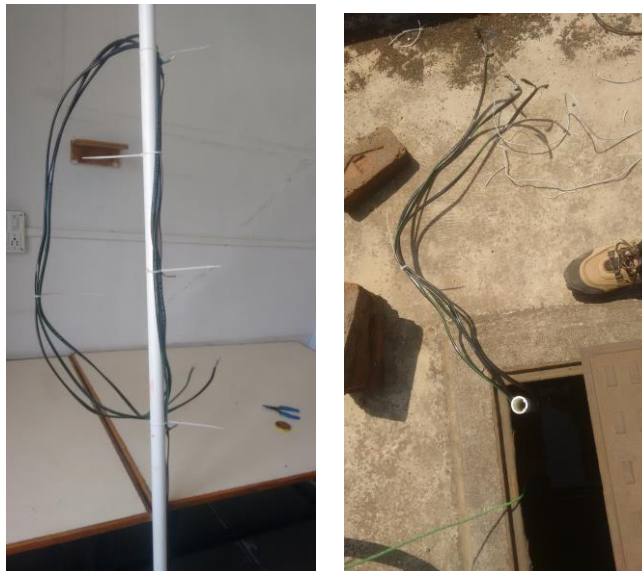
Fig. 3 Designed water level sensor and sensor inserted in water level tank.
