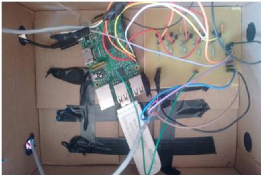
Fig. 4 '3G' dongle connected to raspberry pi
