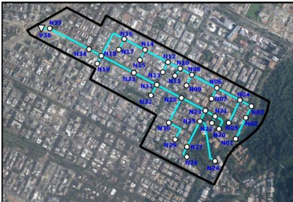
Figure: 4 Representation of the network in the Storm Water Management Model (SWMM) mode
