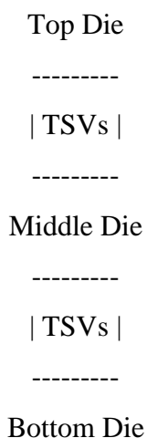
Figure 1: Typical 3D IC stacking with TSVs
