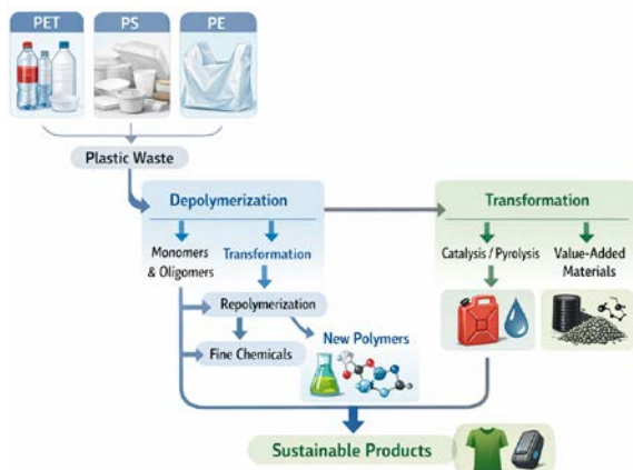
Figure 1 illustrates a schematic overview of chemical recycling and upcycling pathways for common polymers.
