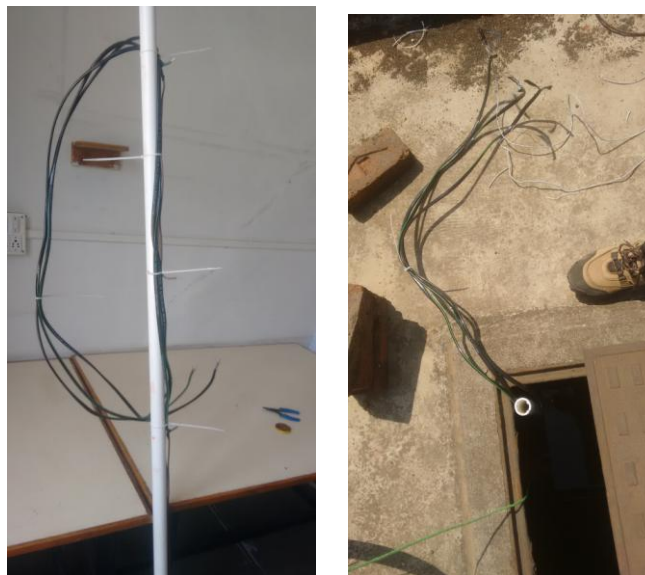
Fig. 3 Designed water level sensors and sensor inserted in water level tank.
