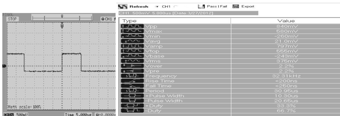
Fig.18: 33% PWM Pulses generated By Microcontroller 89V51
