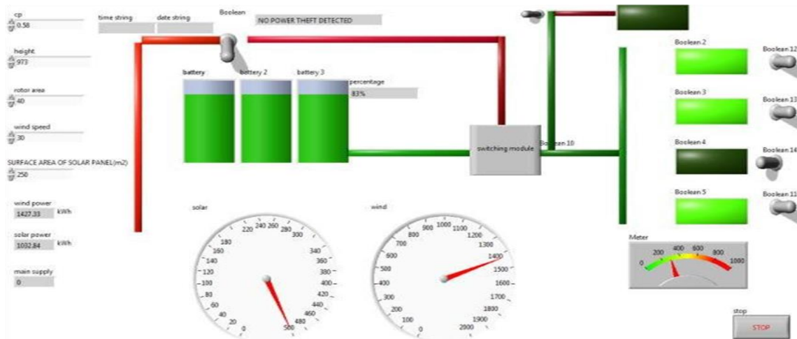
Fig. 4 When battery charges and grid utilizes battery power
