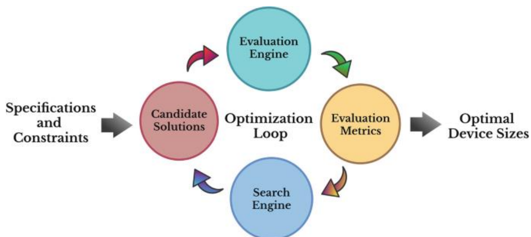
Figure 2: Hybrid EA and AI-Assisted Circuit Optimization
