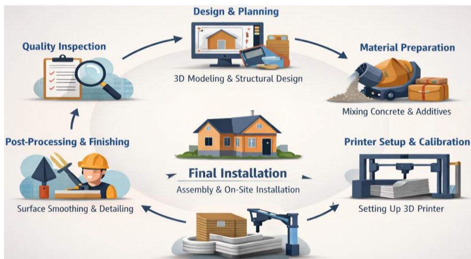
Figure 1: Typical Workflow of Construction 3D Printing
