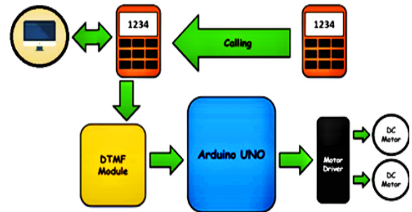
Figure 6: Block diagram of the proposed system
