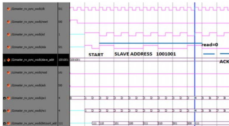
Fig. 6: Simulation Window for I2c Master, Write Mode and Reset Low till Ack is received
