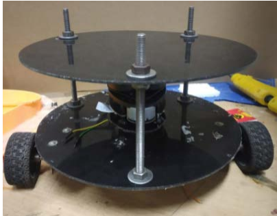
Fig. 7: Frontal view of the SLAM Robot, showing LiDAR Sensor at level 1
