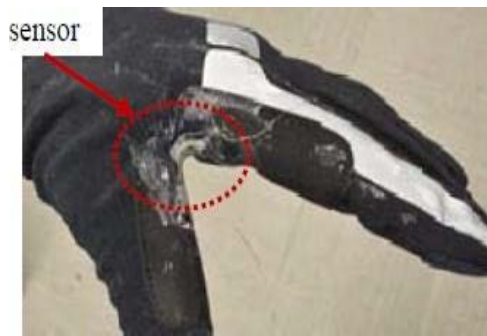
Fig. 7: Strain sensor mounted at pulcrue area to track subtle index finger and palm motion. [2]
